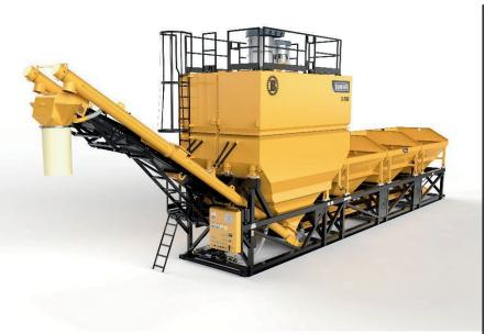
Heavy-duty design with steeper bin angles to reduce material sticking. The B150S boasts high-capacity aggregate bins, and two independent cement powder silos mounted on load cells. The main conveyor features easy access and is closer to the ground level for ease of maintenance. Silo extensions available, contact your local Partner.
