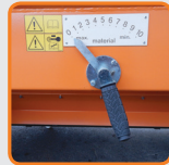
Regulator for the amount of spreading material
