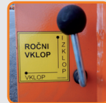
Lever for activation/deactivation of spreader
