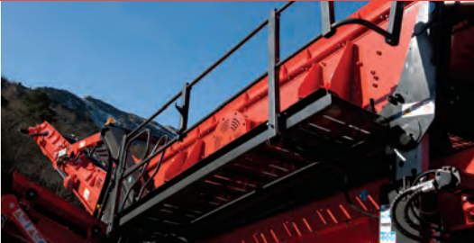
Hydraulically folding maintenance platforms
