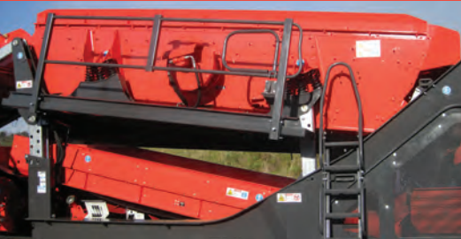
Screen box jack up facility allows easy access
