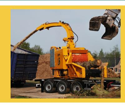
screened prior to chipping.) The 30" upper feed roller with a built-in high-torque Poclain hydraulic motor lifts for full and easy access to the heavy-duty rotor and anvil. The 48" wide x 40" diameter 2-knife or 4-knife drum rotor is engineered with a 6" flame cut pocket design, making it significantly stronger and more durable than anything in the industry.
