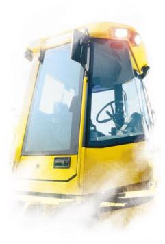
The wide-open, rear mainframe mounted cab allows exceptional visibility. The operator's compartment features a wrap-around tinted windshield which improves operator's peripheral view. Electronic Monitoring System assists the operator with maintenance decisions and improves machine availability.
