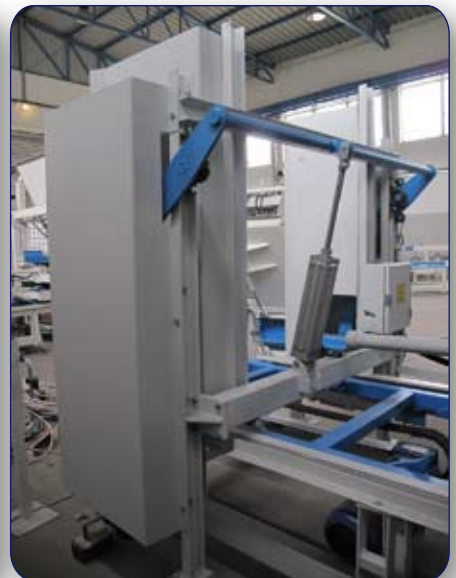
Pallet magazine with speed regulation
