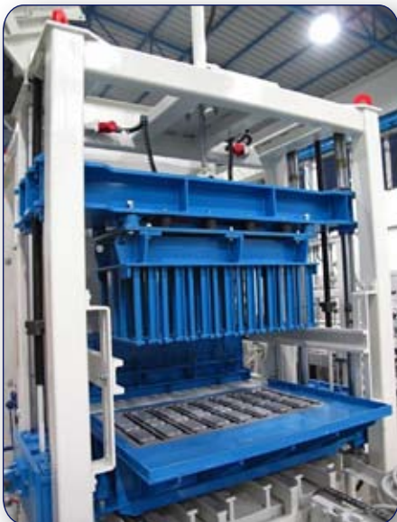
Tamper head bridge
