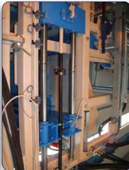
Guide columns and height control
