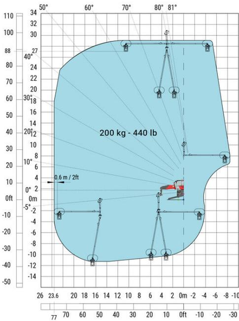
Machine on lowered stabilisers with extensible jib with winch (Metric)
