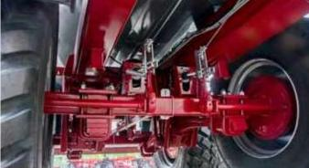
Hydraulically driven rear flap with mechanical blockade and rubber gasket
