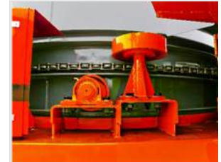
► Press roller combination, ensures tub run smoothly
