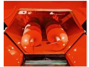
► High efficiency dual augers
