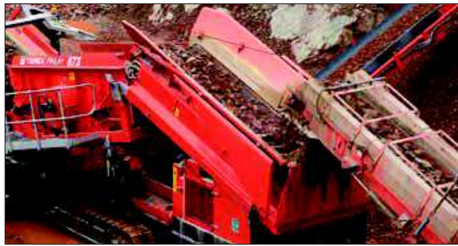
Hopper - Extensions folded for crusher feed
