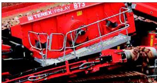
Galvanised Catwalk around Screen
