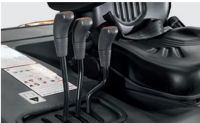
The multi-lever controls give the operator maximum control when using the lifting hydraulic system
