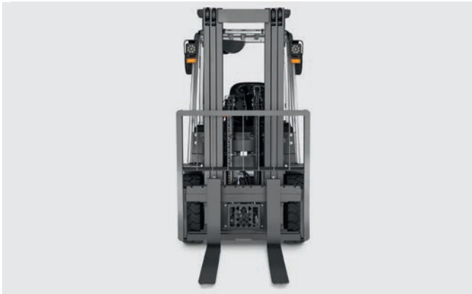
Slim mast profiles ensure a good view around the mast to keep an eye on forks and fork carriage during
