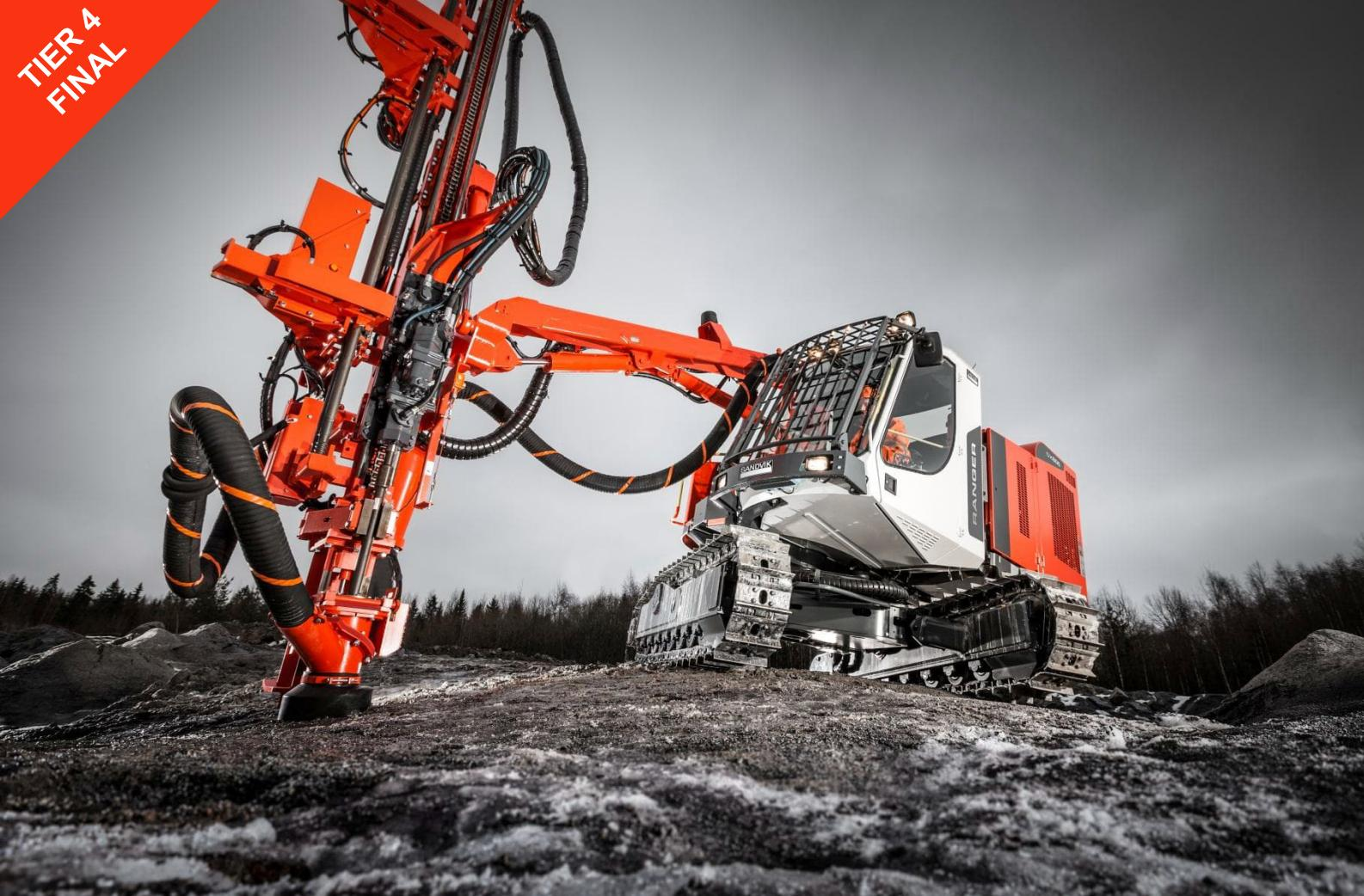
Ranger DX800 is a hydraulic, self-propelled, self-contained, crawler based surface drilling rig equipped with a cabin (F.O.P.S. and R.O.P.S.) and rod handling system.
