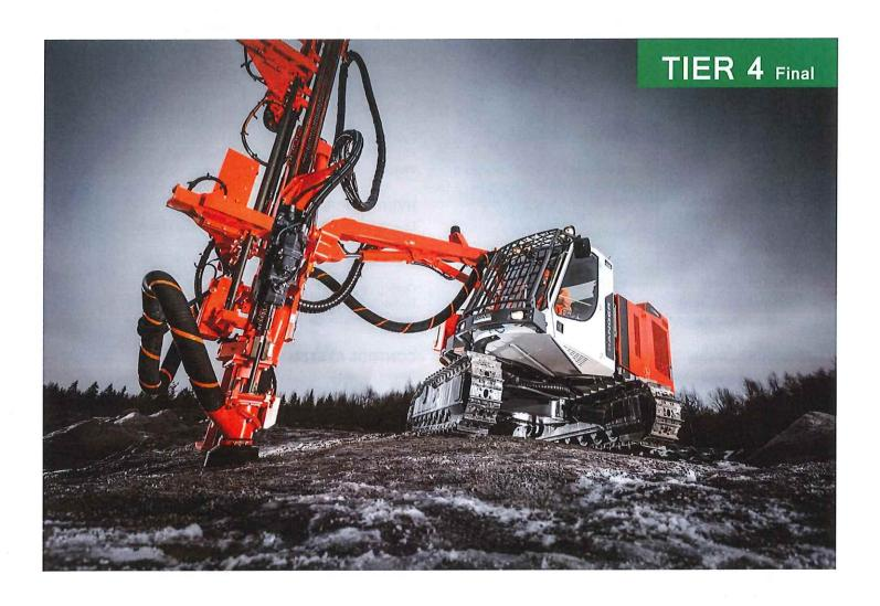
Ranger DX800 is a hydraulic, self-propelled, self-contained, crawler based surface drilling rig equipped with a cabin (F.O.P.S. and R.O.P.S.) and rod handling system.
