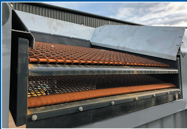
2-DECK VIBRATING SCREEN 1800mm x 1800mm (6' X 6') 3.24m 2 (36ft 2 ) SCREENING AREA PER DECK
