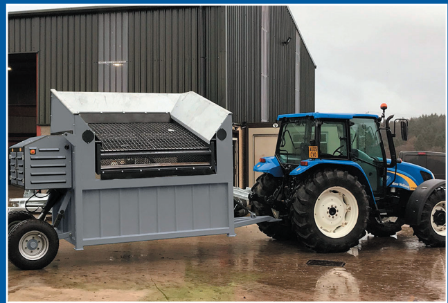
AGRICULTURAL TYRES FOR ON-SITE TRANSPORT ADJUSTABLE DRAWBAR HEIGHT HYDRAULIC JACK LEG AND REAR AXLE
