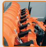
Protection with rigid oscillating links and preloaded spring
