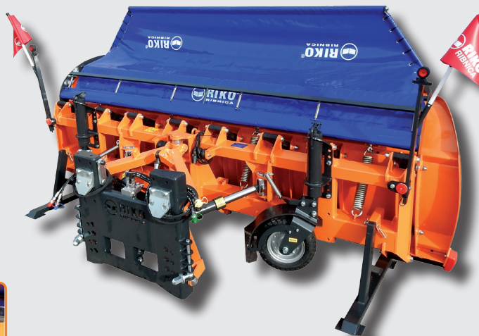
Protection with rigid oscillating links and preloaded spring
