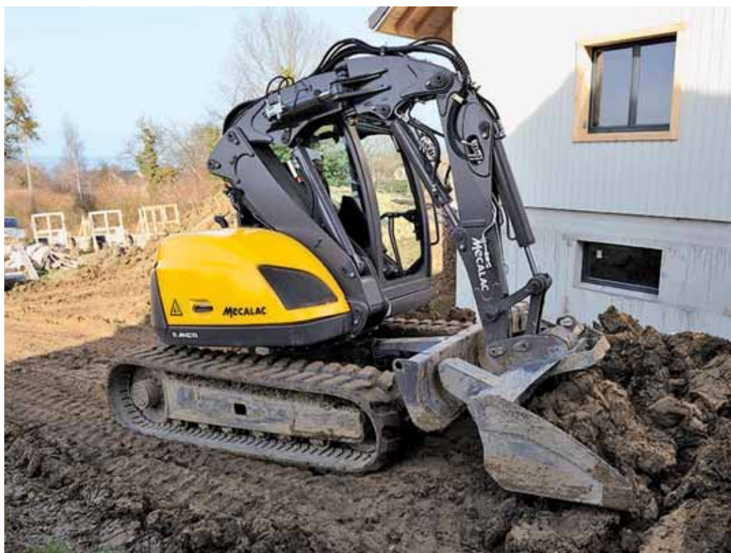
Patented system for recovering the forces induced by the loader bucket pressing on the blade during the loading or stripping phase.
